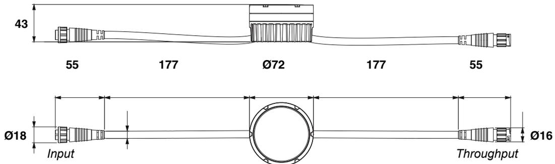
*Direct Dot-to-Dot connection allows up to 0.5 m (19.6 in.) pixel pitch. All dimensions are in millimeters.*
