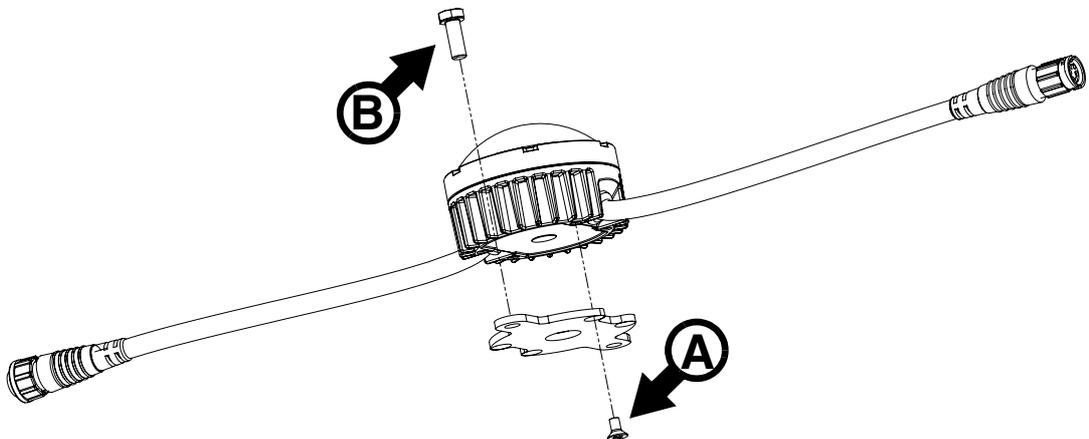
Figure 4: Installing using a mounting plate
