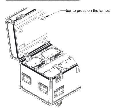
The SiP insert must be inserted into a Flightcase for 8x MAC One: P/N: MAR-91515058
